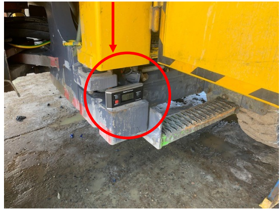
Lengthways calibration Shown. fig. 3
